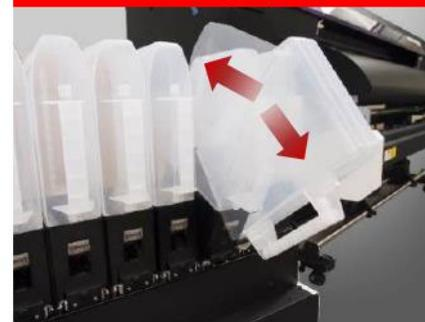
The new ink supply system allows for easy maintenance of inks that require frequent shaking for consistency.
