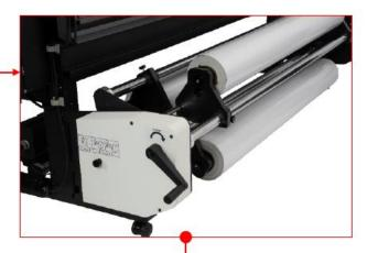
**NEW:** ROLL CHANGE SYSTEM Accepts up to 3 rolls for changing the print media quick and easily within a seconds
